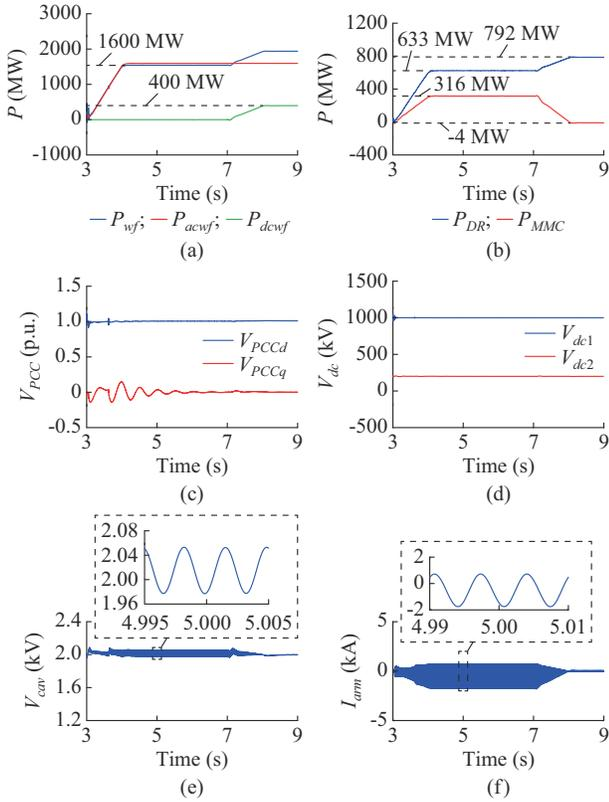
Fig. 9. Simulation results of proposed integration scheme under normal operation. (a) OWF power. (b) Active power of MMC1 and two DRs. (c)  $dq$ -axis components of PCC voltage. (d) DC voltage. (e) Average SM capacitor voltage of phase A of MMC1. (f) Upper arm current of phase A of MMC1.
