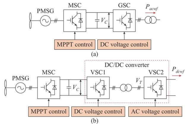
Fig. 2. Topology and control strategy of AC and DC WTs. (a) AC WT. (b) DC WT.
