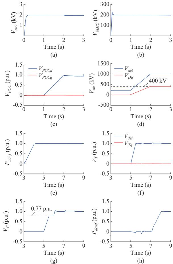
Fig. 8. Simulation results of proposed integration scheme during startup process. (a) Average SM capacitor voltage of MMC1. (b) DC voltage of MMC1. (c)  $dq$ -axis components of PCC voltage. (d) DC voltage of onshore hybrid MMC and DRs. (e) Power of AC wind farms. (f)  $dq$ -axis components of VT. (g) Capacitor voltage in DC WTs. (h) Power of DC wind farms.
