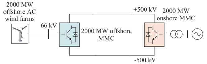
Fig. 6. Topology of AC collection and MMC-HVDC transmission integration system.
