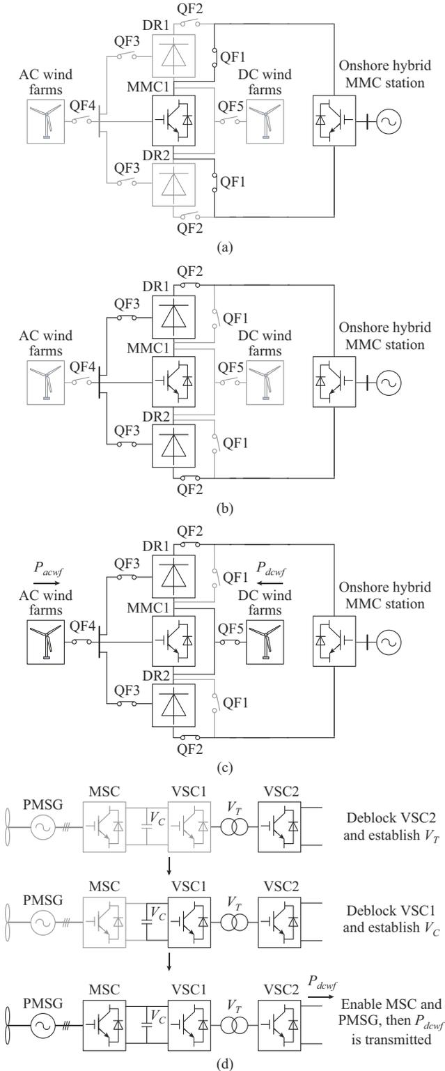
Fig. 7. Startup process of integration system. (a) Stage 1. (b) Stage 2. (c) Stage 3. (d) Startup process of DC WT.
