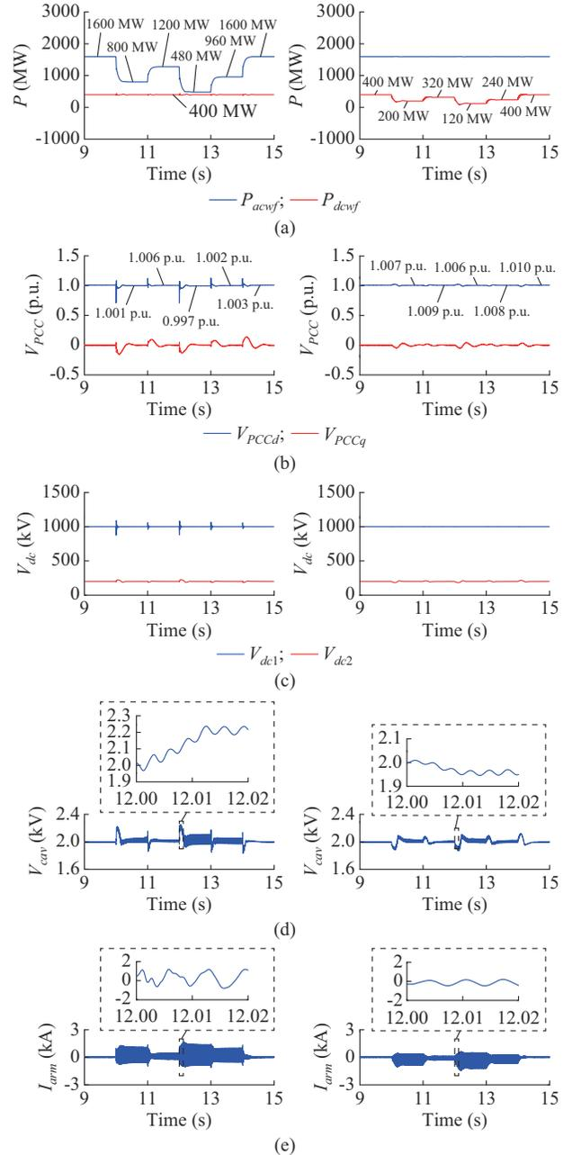
Fig. 10. Simulation results of proposed integration scheme under wind power fluctuations. (a) OWF power. (b)  $dq$ -axis components of PCC voltage. (c) DC voltage. (d) Average SM capacitor voltage of phase A of MMC1. (e) Upper arm current of phase A of MMC1.
