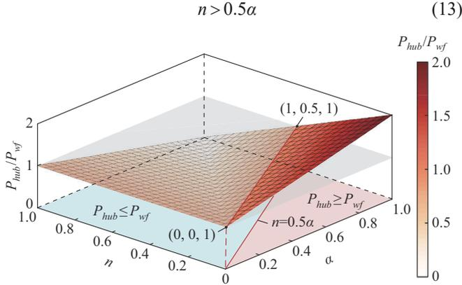
Fig. 5. Power ratio between  $P_{hub}$  and  $P_{wf}$  versus different power ratio  $\alpha$  and DC voltage ratio  $n$ .
