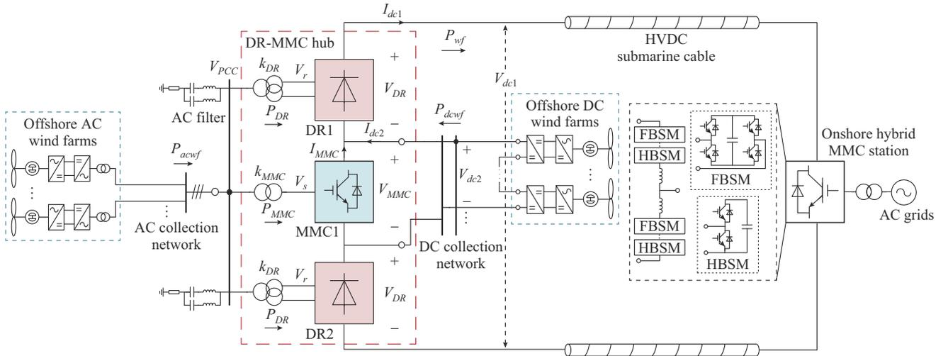
Fig. 1. Topology diagram of proposed hybrid AC/DC collection and HVDC system for large-scale offshore wind power integration.
