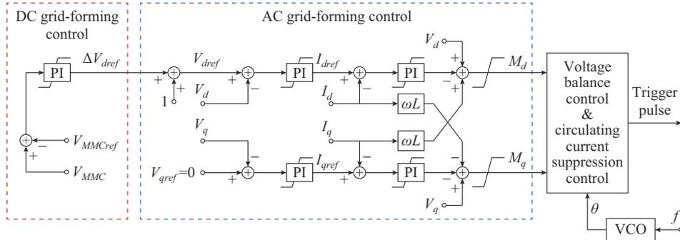
Fig. 4. Dual grid-forming control of offshore MMC1.
