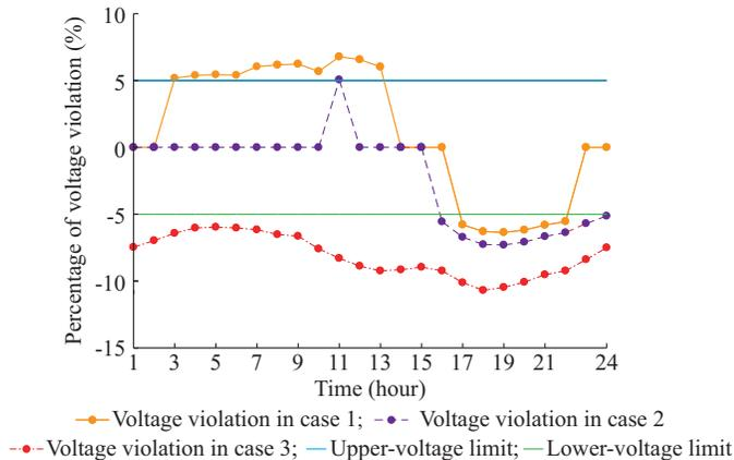
Fig. 4. Voltage violation of IEEE 33-bus distribution network in cases 1-3.
