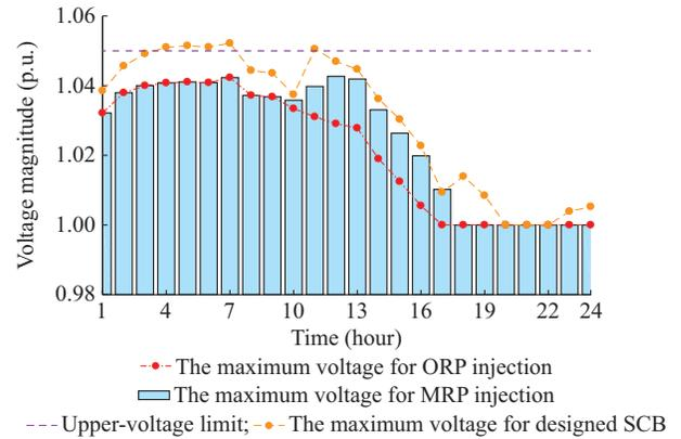
Fig. 8. Hourly values of the maximum network voltage.
