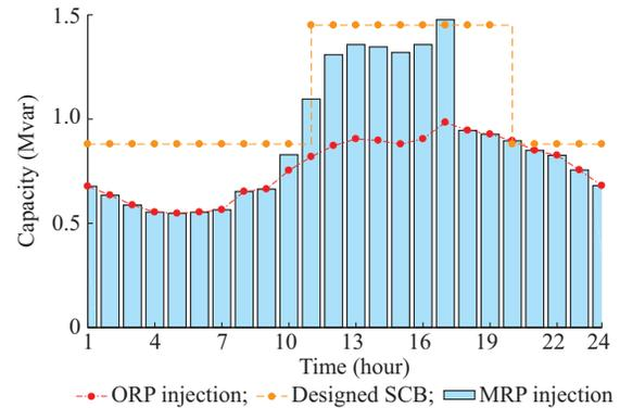
Fig. 5. Hourly values of reactive power injection for optimal curve, modified curve and designed SCB.
