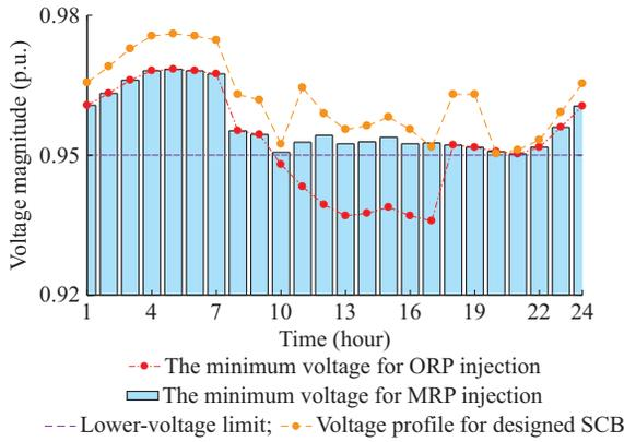
Fig. 6. Hourly values of the minimum network voltage.
