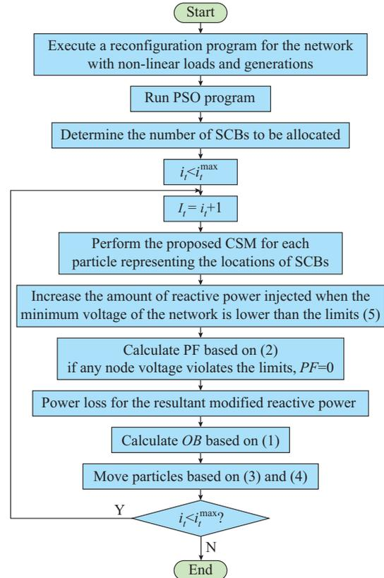
Fig. 2. Flowchart of instruction of proposed CSM.
