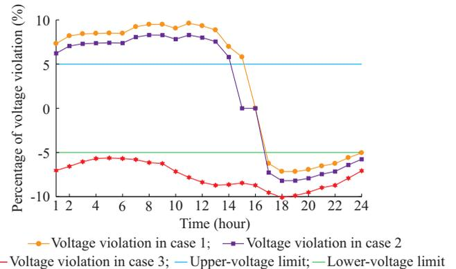
Fig. 11. Voltage violation of modified IEEE 69-bus distribution network in cases 1-3.
