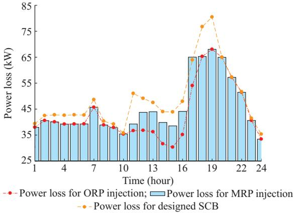
Fig. 7. Hourly values of power loss difference.
