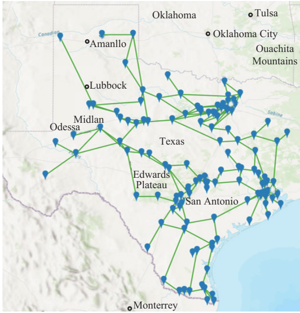
Fig. 1. High-voltage backbone transmission network of TX-123BT system.
